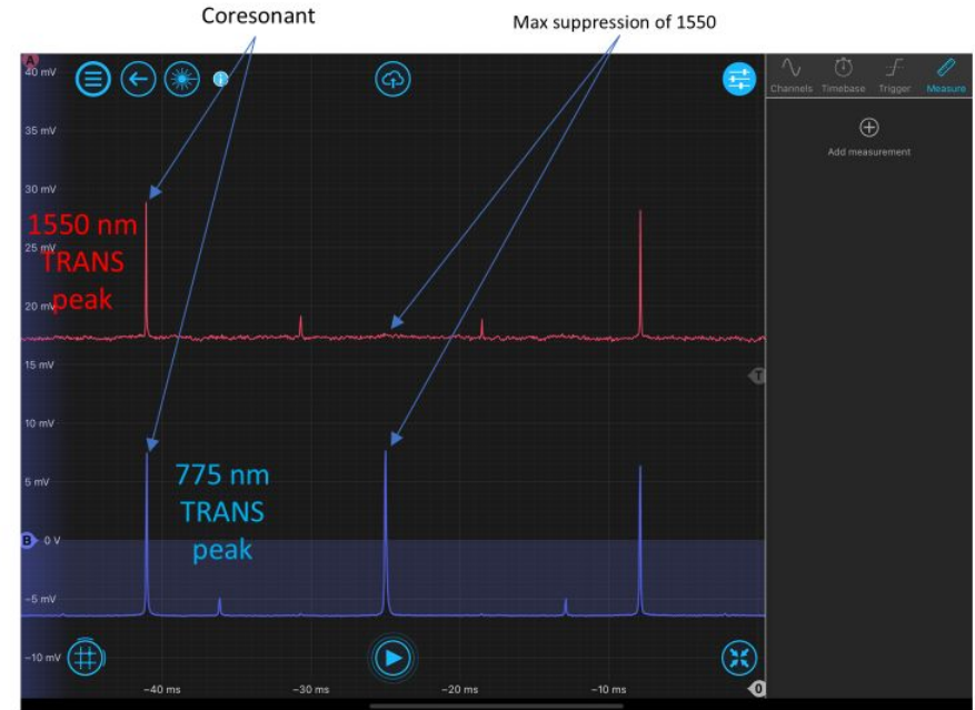
Scan using laser over full a FSR
