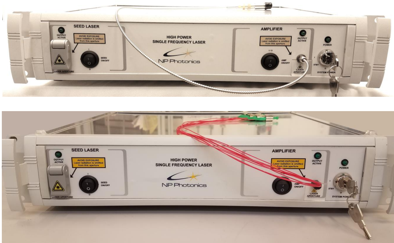
Figure 5.1 Front Panel of the RFLPXA (multiple output options shown)
